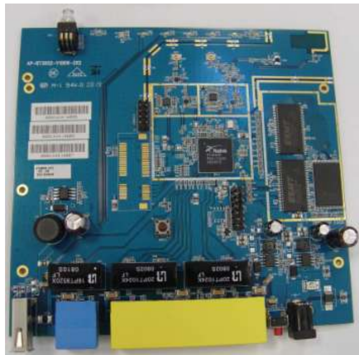
Figure 2 The RT3052 Demo Board
