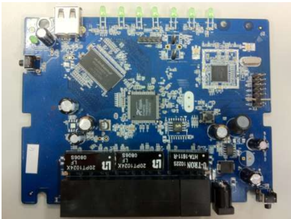
Figure 6 The RT6855 Demo Board
