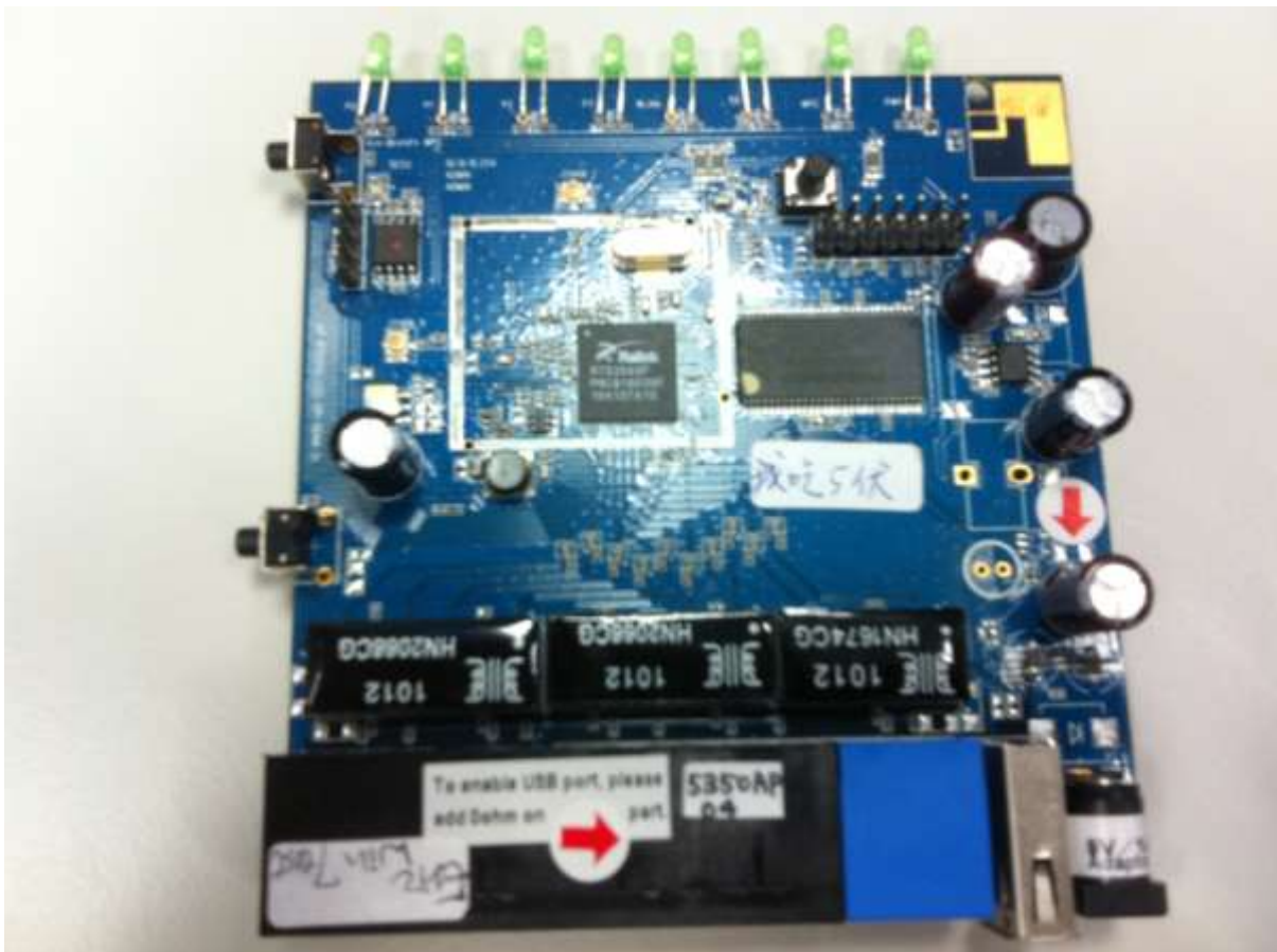
Figure 5 The RT5350 Demo Board
