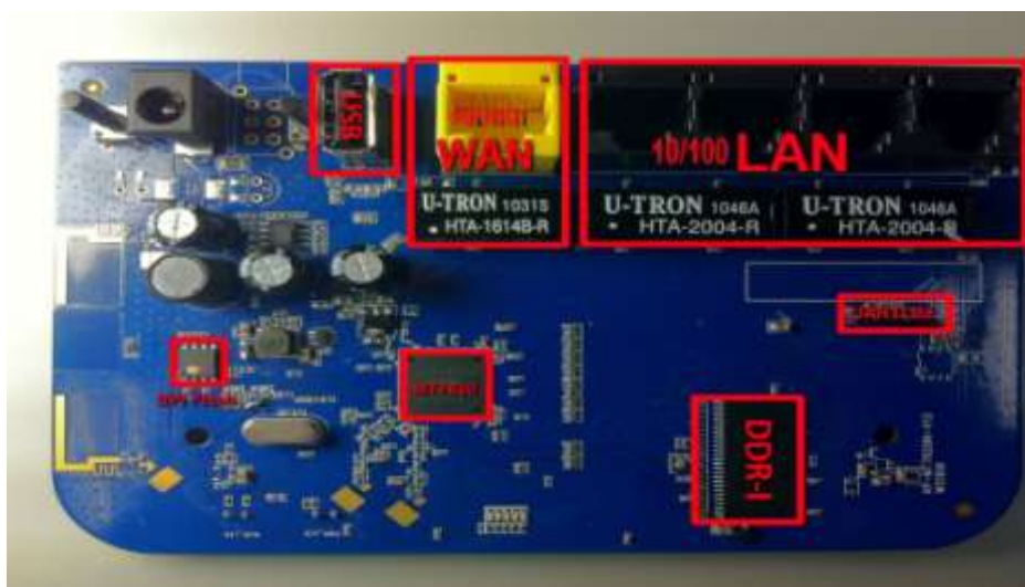
Figure 8 MT7620N Demo Board
