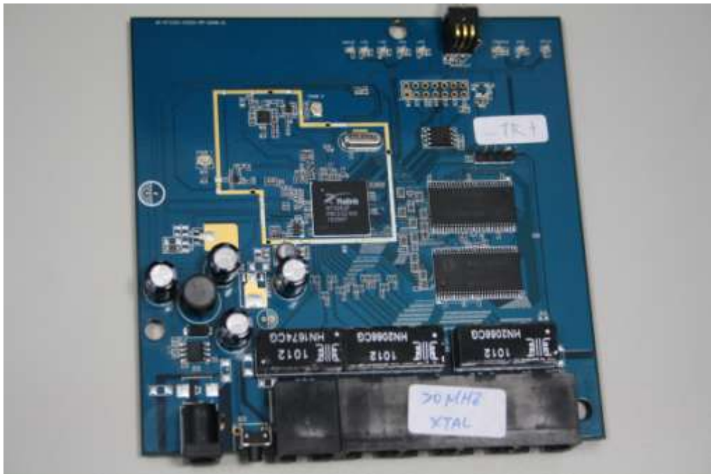
Figure 4 The RT3352 Demo Board
