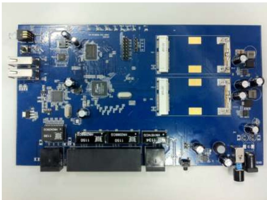
Figure 7 The RT6856 Demo Board
