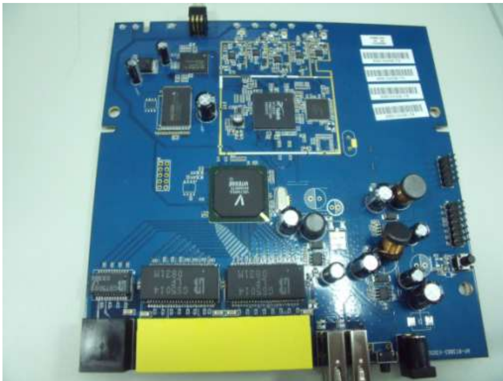
Figure 3 The RT3883 Demo Board
